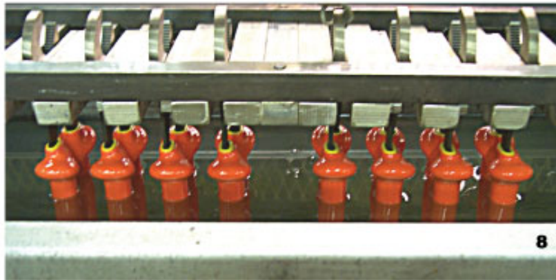
1 Screwdriver adhesion test 2 Wrench adhesion test 3 Flammability test 4 Impact test 5 Screwdriver test (close up) 6 Indentation test 7 Completed tool test 8 Dielectric test
